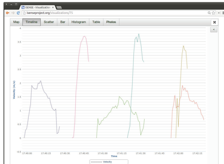
Figure 6. Timeline visualization of students' data walks, showing velocity vs. time. Some of the data are overlaid because students were simultaneously recording their walks on two different devices; the graph shows all of their data together, regardless of which device initially recorded it.
